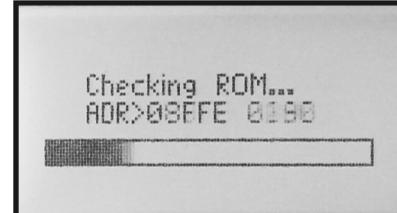
1. When first plugging in the Inno-Clean+ control unit to a power source the control unit will go through an initialization process which will require the operator to enter 4 desired settings.
