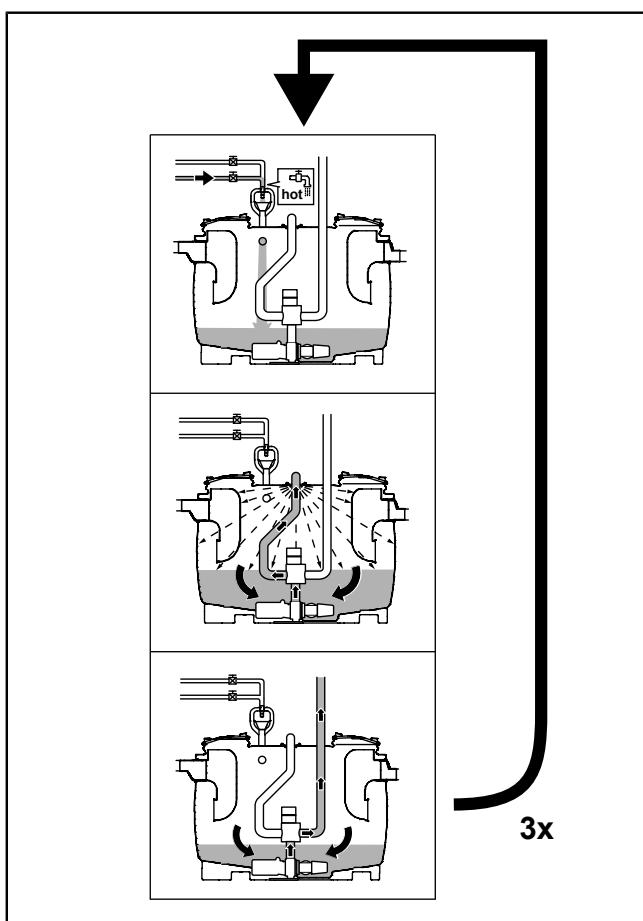
① The sequence of the individual program steps with running time recommendations is given in the table below.
